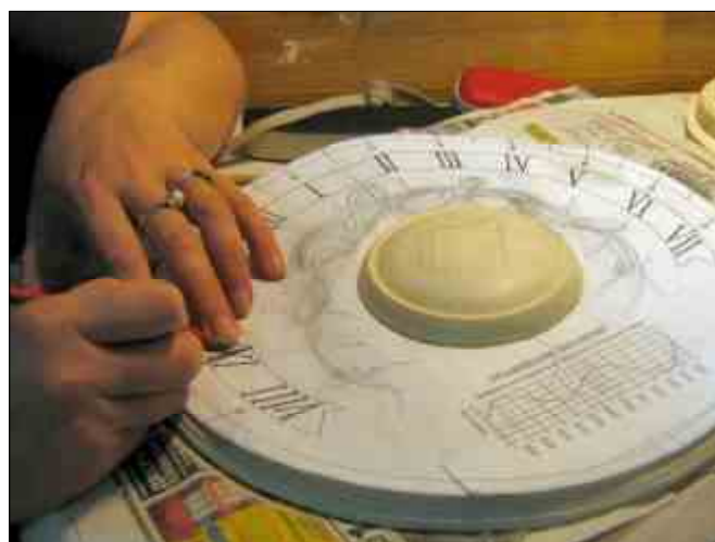
Fig. 2. Transferring the dial drawing.
